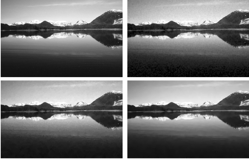
Fig. 1. One image from the dataset in [15], and its denoising results (noise level \sigma_\eta = 35 ). Top left: original image. Top right: K-SVD (PSNR = 31.01, SSIM = 0.857). Bottom left: BM3D (PSNR = 33.16, SSIM = 0.923). Bottom right: Fused K-SVD algorithm (PSNR = 33.16, SSIM = 0.940). Note the artefacts in the single scale patch based methods.
