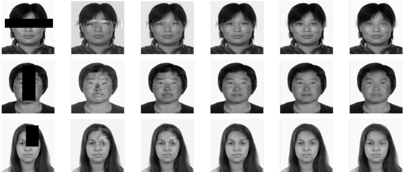
Fig. 1. Inpainting of the image on the left column, for increasing values of \lambda (from left to right) in the range [0.05, 50] , with Trainlets.
